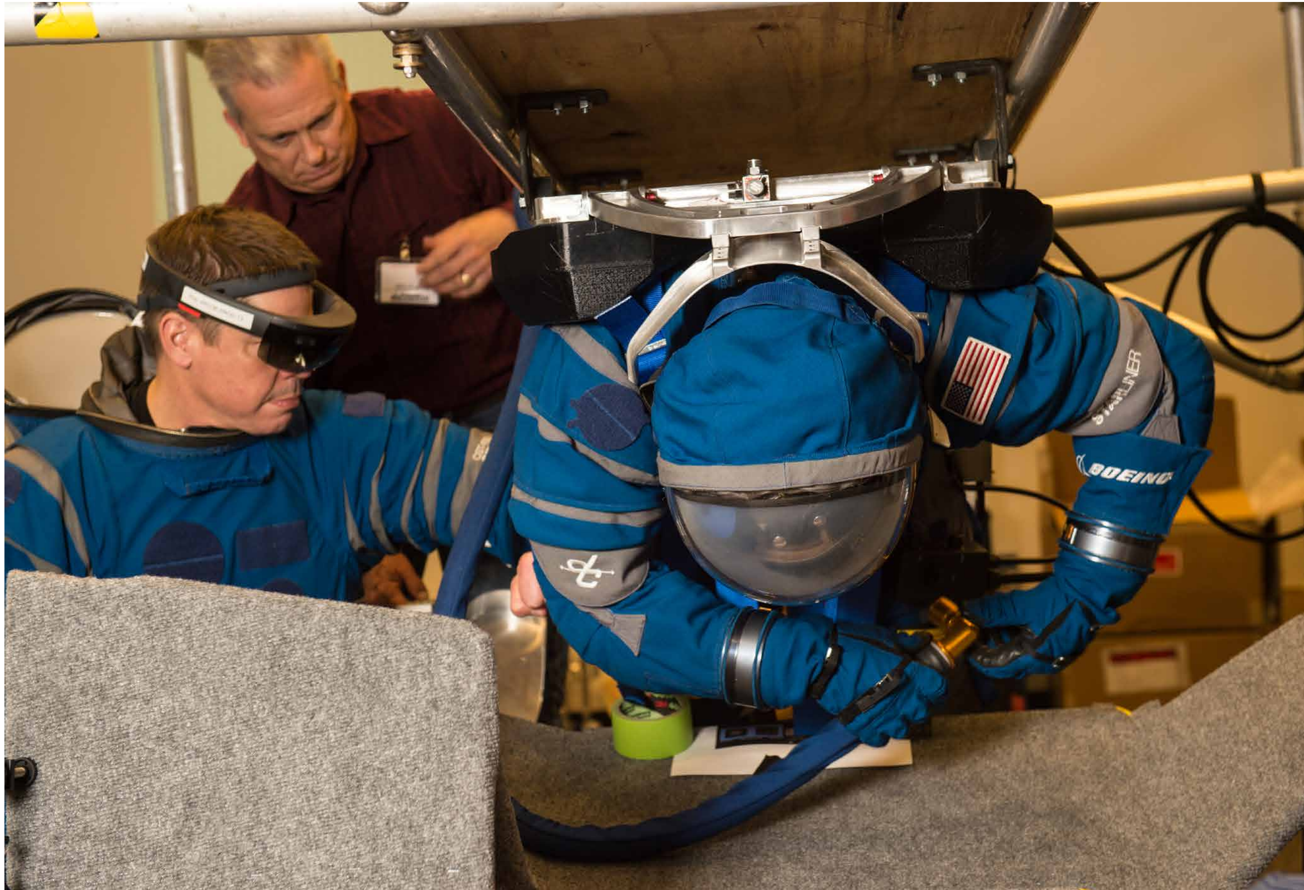
NASA's Commercial Crew Program astronauts, wearing spacesuits and augmented reality headsets, rehearse returning to Earth from the International Space Station during recent testing at Boeing's Extended Reality Laboratory in Philadelphia. The astronauts are seated upside down so they can practice releasing their seat harness and moving to the side hatch of the Starliner without assistance. The astronauts wearing the mixed reality gear see a digital version of the interior of the Starliner as it would look in the real-life scenario while interacting with the environment around them. Both Boeing and SpaceX have been working with the astronauts training to fly the test missions to the International Space Station. Photo credit: Boeing
