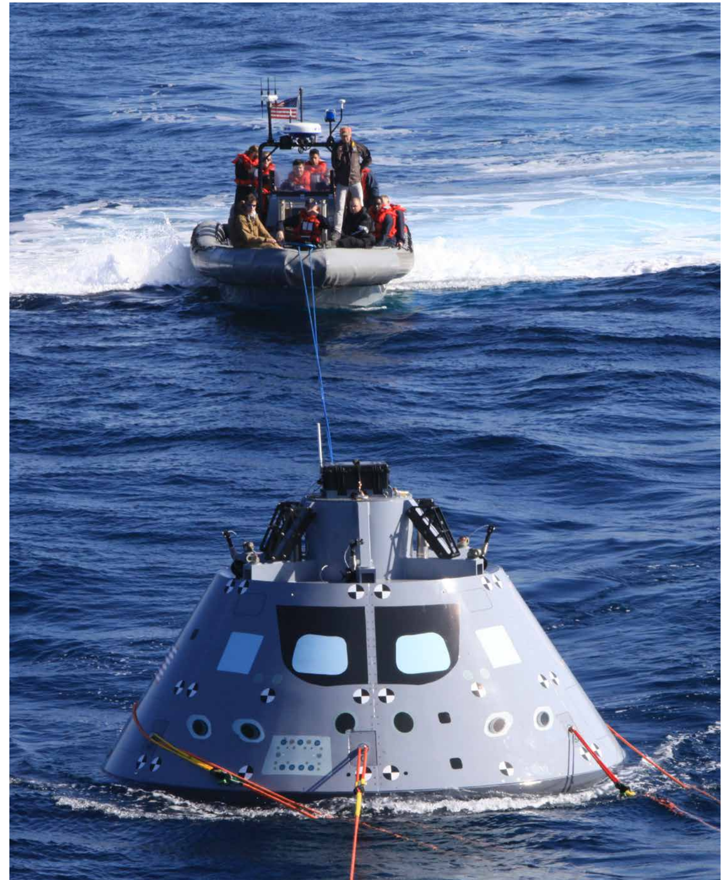
As part of Underway Recovery Test 6, the Orion test article is pulled in by a winch line at the rear of the USS Anchorage's well deck that brings the capsule into the ship, along with four manned LLAMAs (Line Load Attenuation Mechanism Assembly) that control the capsule's side-to-side movement and a tending line attached to a rigid hull inflatable boat for controlling Orion's movement behind the ship. The testing with Kennedy Space Center's NASA Recovery Team and the U.S. Navy will provide important data that is being used to improve recovery procedures and hardware ahead of Orion's next flight, Exploration Mission-1, when it splashes down in the Pacific Ocean. Photo credit: NASA/Bill White
